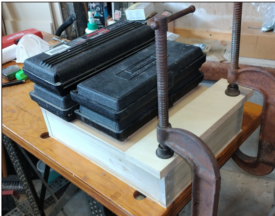
Sanding stick trick; Gluing up the top & bottom (note slight overhang).
