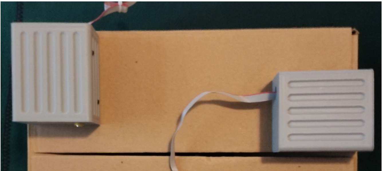
Figure 2. Here the volume box is rotated 90 degrees counterclockwise which might help to minimize magnetic interaction, and the hot end of the volume coil is then positioned nearest to the volume antenna. Volume loop antenna mount clearance could be a problem.
